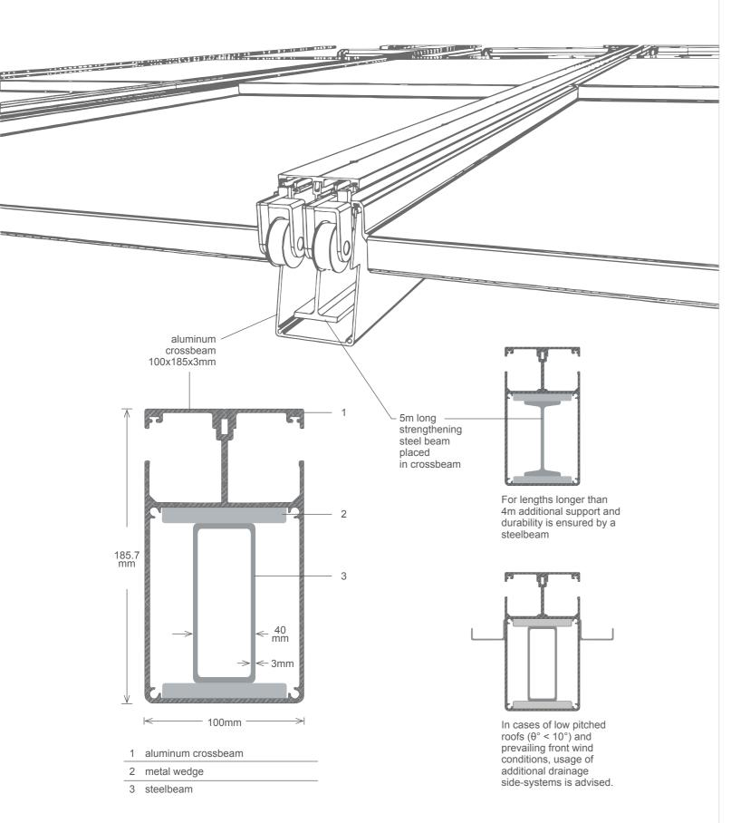
Salinox's sliding roofs use a heavy type of aluminum profile specially designed to accommodate an internal drainage system. Water flows off the panels to the peripheral drainage, ensure perfect functionality and watertightness even under bad wheather conditions.
