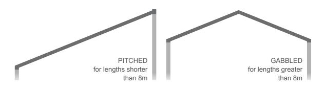
In cases where the construction exceeds 8m in length, the roof cannot be pitched, it has to be turned into a gabbled design to ensure safety and adhere to regulation.
