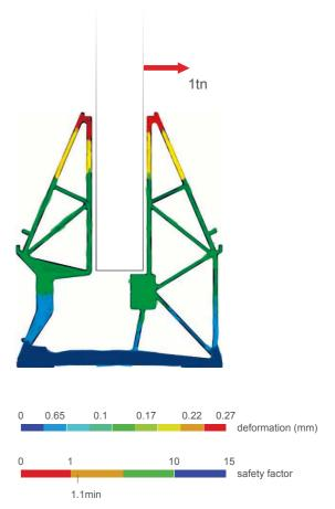
Strain load on 50cm mount with 1ton (,000Nt) vertically on glassboard holding surface.
