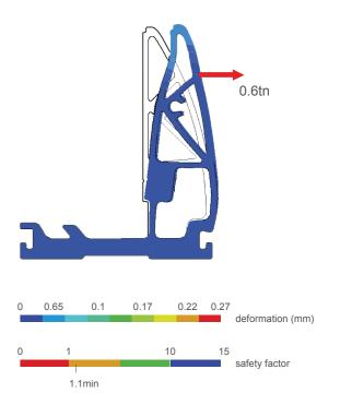
Strain load on 50cm mount with 0.6ton (6,000Nt) vertically on glass-board holding surface.
